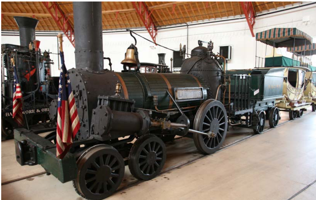
Photo Left: B&O 4-2-0 "Lafayette" was the first engine to utilize a horizontal boiler
