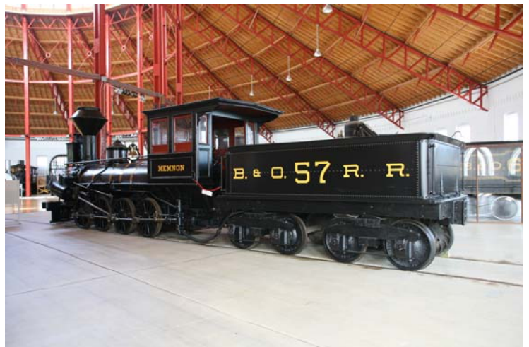
Photo Above: B&O 0-8-0 #57 “Memnon” has blind (flangeless) center drivers built in 1848. This same technique was used years later by Lionel to allow larger engines to run on 031 track!
